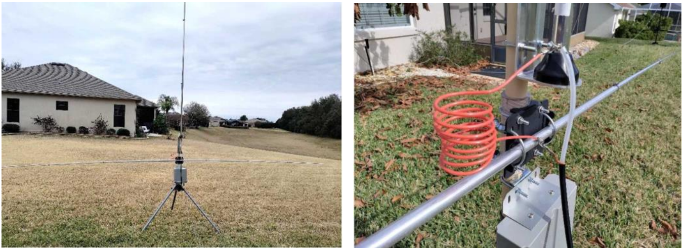
Figure 1: My homemade V8 Vertical Dipole
