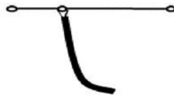
2. Off Center Fed Half-wave Dipole (G5RV)
