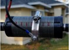
Here is the modified Buddipole / BuddiStick tuning collar. If you are configuring for vertical, only one is needed. For the Buddipole in the conventional dipole configuration, you would need two.
