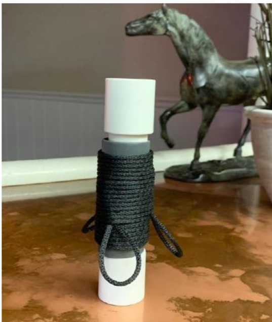
(Below) Finished project! Efficient high guy point that requires NO drilling, no metal fasteners to scratch fiberglass pole and..... it cost a dollar to make it!!
